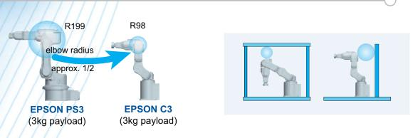
The enhanced new slim body and compact wrist design of the C3 allows for greater motion range and less mechanical restrictions. Designed for maximum performance, C3 robots have a good combination of high quality components for light weight arms and high rigidity. Furthermore, user bolt patterns have been added on each axis, for easy mounting of peripheral equipment. C3 robots are the compact footprint champion and the most flexible 6 axis robots available in the market today.
